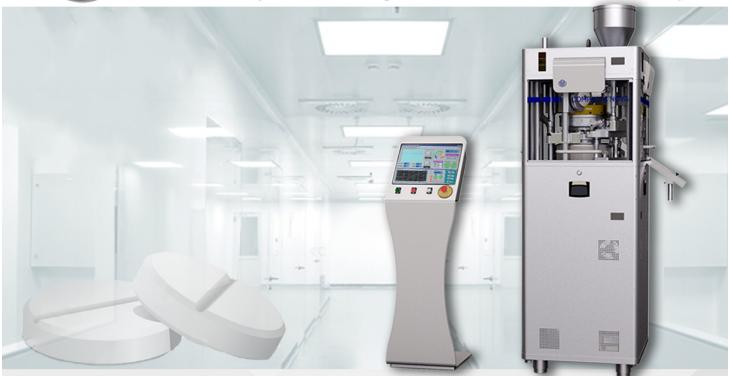
The Compacta Nova is a rotary tablet press designed for a medium scale single-layer tablet production. It has a standard turret head removal system that allows a quick tooling change, obtaining a significant time reduction in equipment cleaning and preparation. Its solids structure with transparent polycarbonate upper doors allows access and visibility into the work area.
