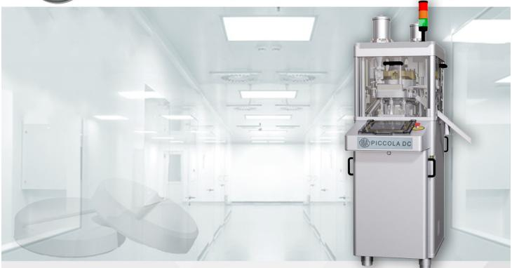
This rotary tablet press was designed to represent the production conditions of pharmaceutical units formed by two layers. These layers can be made of granules or product of equal or different characteristics and in small batches, according to the development needs for new products.
