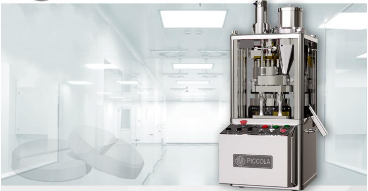
The PICCOLA CLASSICA is a rotary tablet press intended for implementation in the research and development area, and it is designed for pilot plants and/or small production batches. Its settings allow operating with one to ten sets of punches placed in the turret head. Punches and dies conform to the international TSM or EU (B/D) standards.
